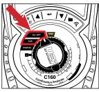
Rotate rotary dial to 02/Eff or C0/C02 setting.
